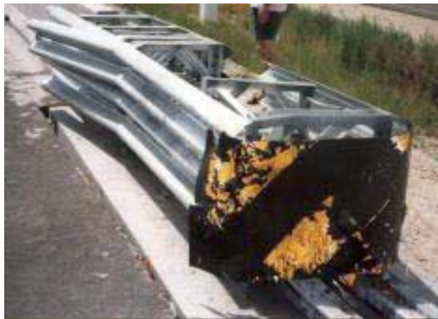
Damaged TRACC in Boise, Idaho
